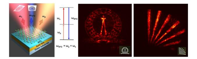
From left to right: Schematic of the nonlinear optical mirror used for upconversion imaging. Energy diagram showing the sum frequency generation process used for up-conversion. Representative up-converted images of IISc logo and spokes where the object pattern at 1,550 nm is upconverted to 622 nm wavelength. Credit: Jyothsna KM
