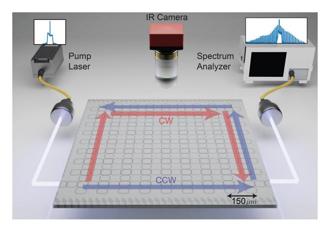
A schematic of the new experiment. Incoming pulsed laser light (the pump laser) enters a chip that hosts hundreds of microrings. Researchers used an IR camera above the chip to capture images of light circulating around the edge of the chip, and they used a spectrum analyzer to detect a nested frequency comb in the circulating light. Credit: C. Flower
