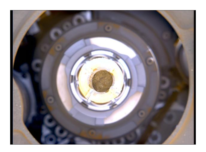
This image shows the rock core from "Berea" inside inside the drill of NASA's Perseverance Mars rover. Each core the rover takes is about the size of a piece of classroom chalk: 0.5 inches (13 millimeters) in diameter and 2.4 inches (60 millimeters) long. Credit: NASA/JPL-Caltech/ASU/MSSS
