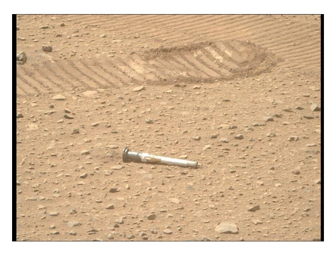
A sealed tube containing a sample of the Martian surface collected by NASA's Perseverance Mars rover is seen here, after being deposited with other tubes in a "sample depot." Other filled sample tubes are stored within the rover. Credit: NASA/JPL-Caltech
